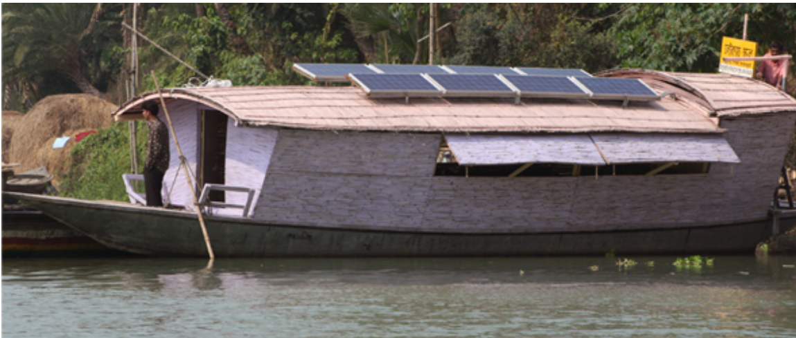
A Shidhulai Swarnirvar Sangstha solar powered school boat. (Image: Shidhulai Swarnirvar Sangstha)
